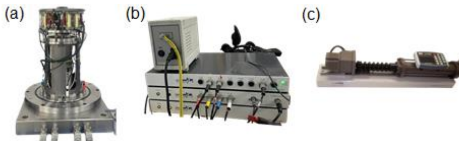
Fig. 2 Resonant Column Apparatus (RCA): (a) RCA device, (b) system hardware, (c) back pressure
